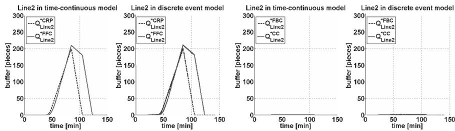
**Figure 4:** Buffer in Production Line 2 in time-continuous and discrete event model
