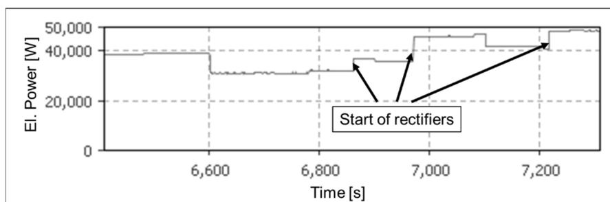
**Figure 4:** Load profile of the total plating line
