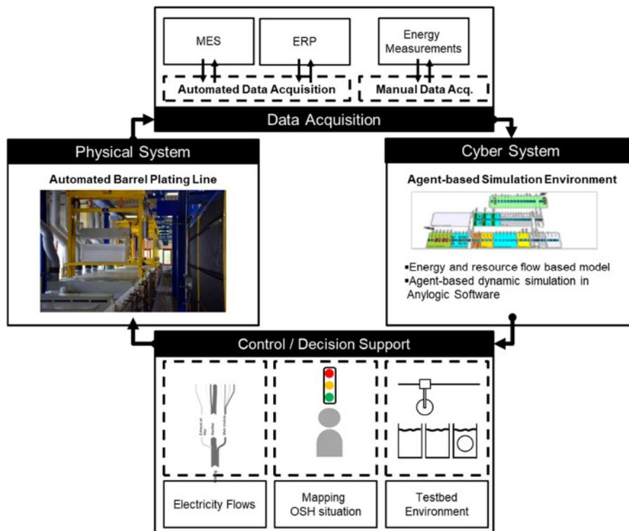
**Figure 2:** Integration of simulation as cyber system into a CPPS
