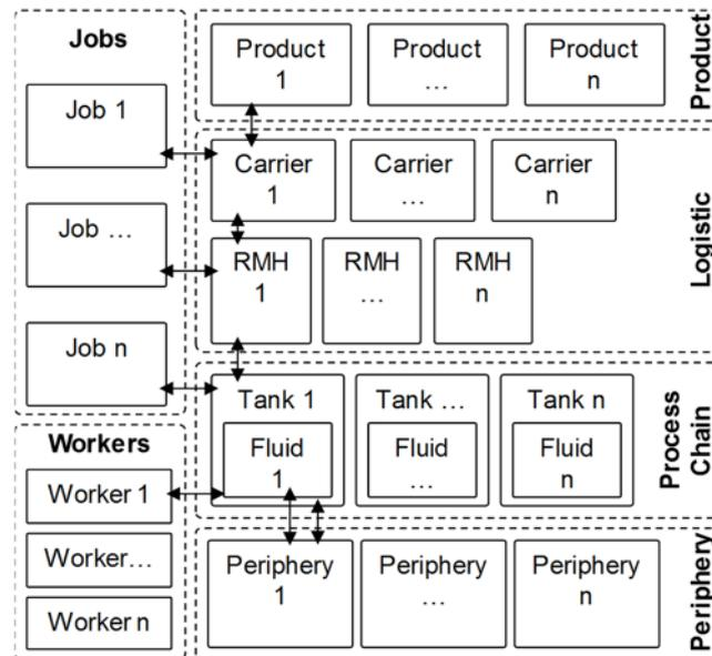
**Figure 3:** Structure of the simulation model
