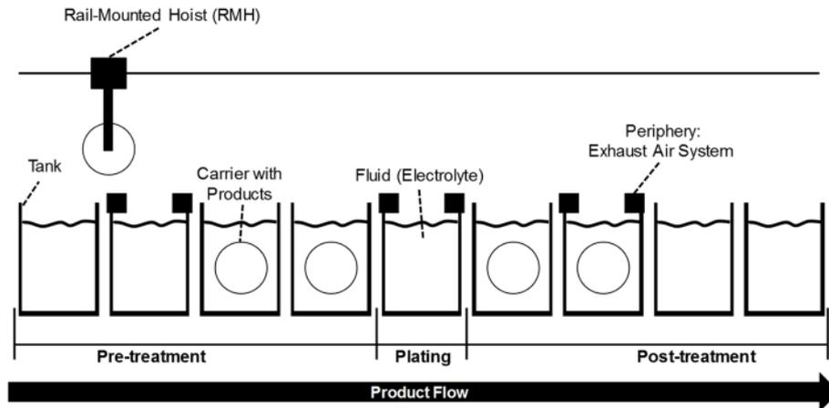
**Figure 1:** Schematic overview of an industrial automated electroplating line
